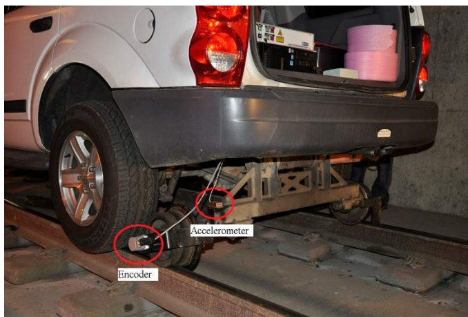
Figure 112 Installation of wheel encoder and accelerometer.
