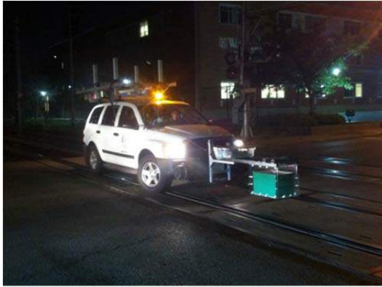
UVM GPR system mounted on the railroad vehicle
