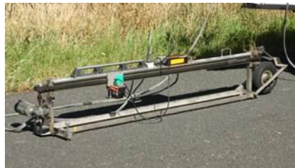
Figure 6. SLP (Stationary Laser Profiler)
