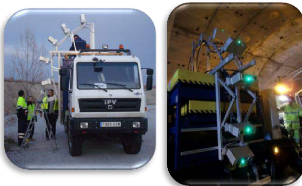
Figure 3 - LTSS Mounted on an All-terrain Vehicle
