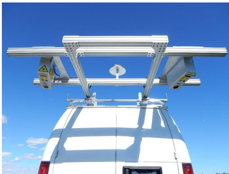
Photo of the 3D laser profilers (LCMS) and INS system on the survey vehicle.
