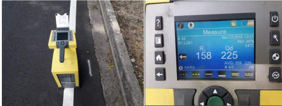
Fig. 6 Retroreflectometer result shown real-time
