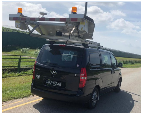
Fig. 3 LCMS-2 Survey Vehicle with two sensors
