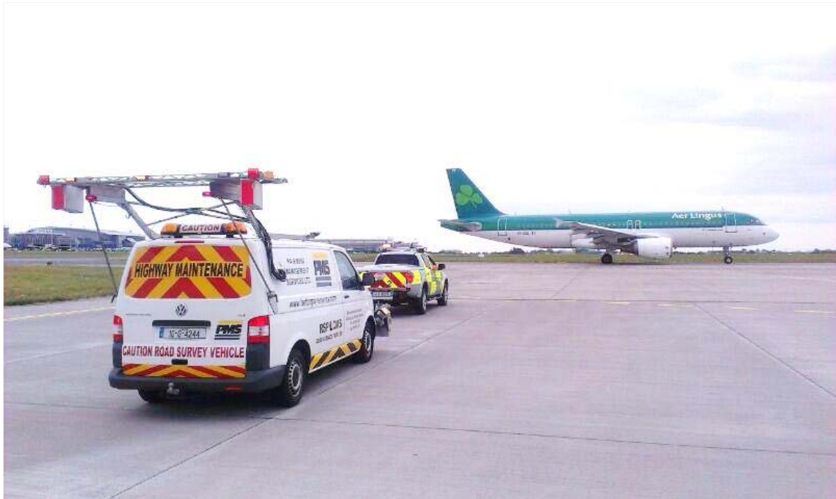
FIGURE 1 High-Speed LCMS Survey Vehicle at Dublin Airport.
