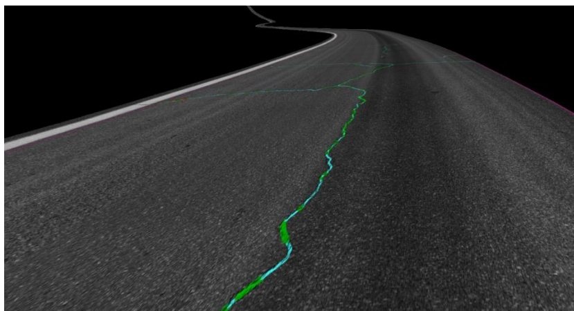
Figure 8 : 3D view of the road with cracks from Aigle 3D measurements
