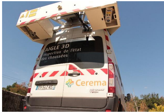
Figure 4 : Aigle 3D inspection vehicle developed by Cerema and equipped with LCMS© sensors.
