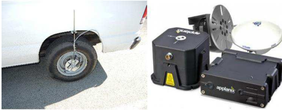
Figure 3: Photo of Wheel Encoder and INS Including GNSS Receiver, Antenna and IMU
