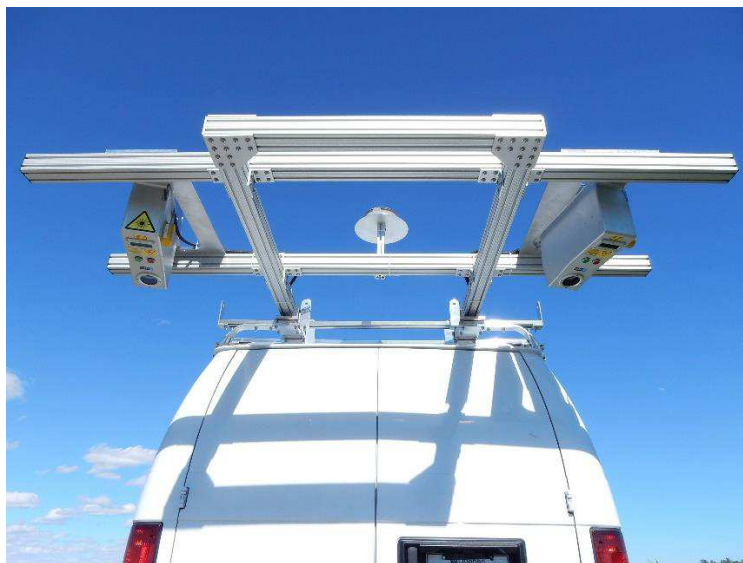
Figure 2: Photo of the 3D laser profilers and GPS Antenna on the survey vehicle
