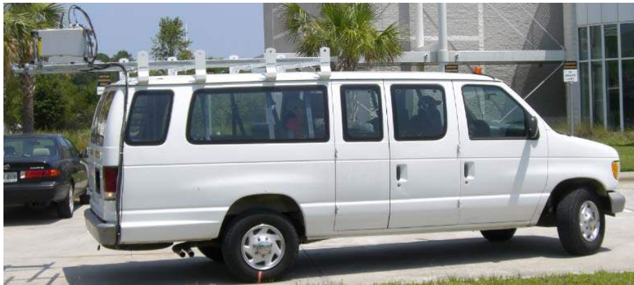
Figure 2 The sensing van for collecting faulting data.
