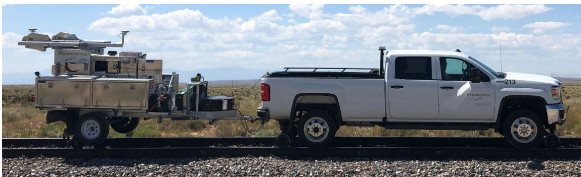
Figure 4. Hi-rail Truck Pulling Test Trailer Equipped with LRAIL System
