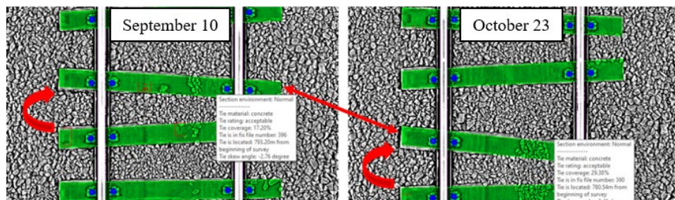
Figure 34. Example of Crosstie Skew Angle Increase
