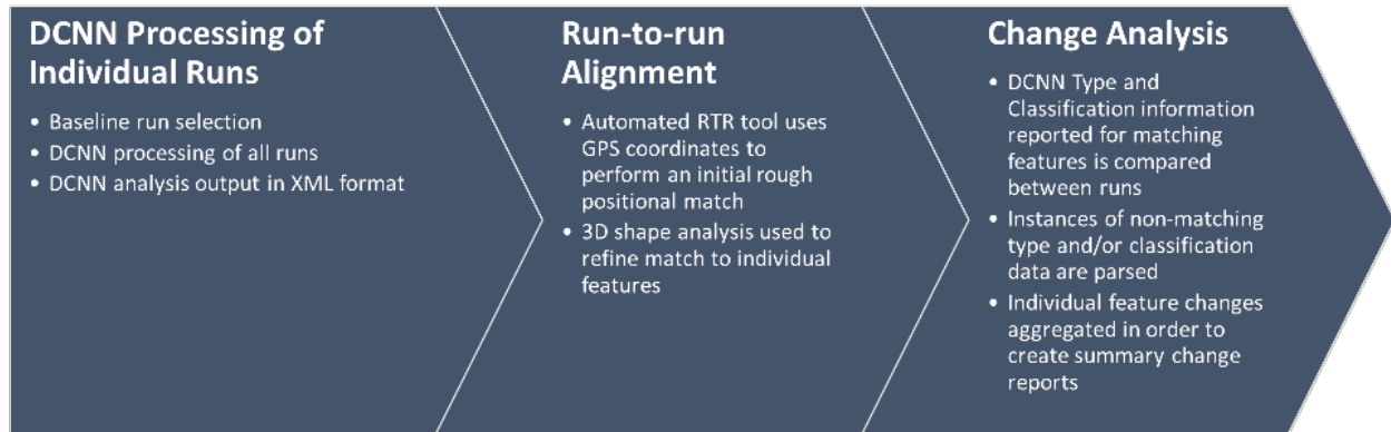
Figure 14. Change Detection Process Flow
