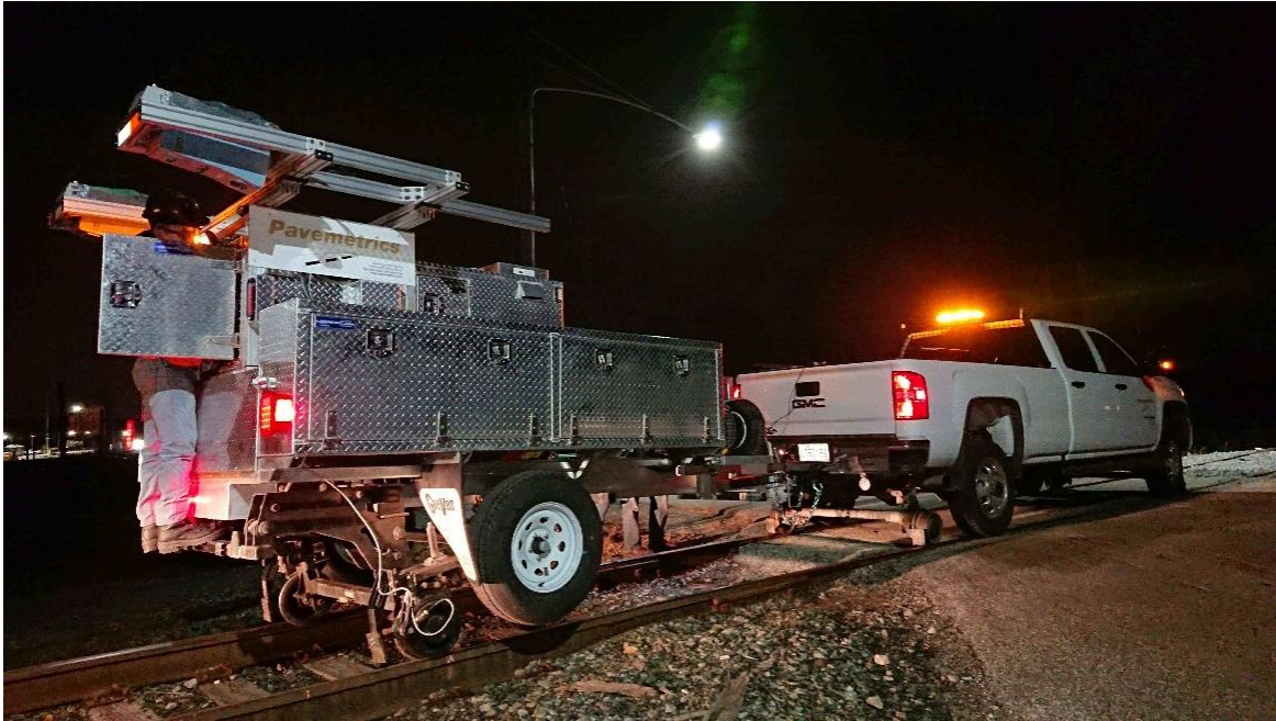
Figure 5 - LRAIL Self-contained Test Trailer
