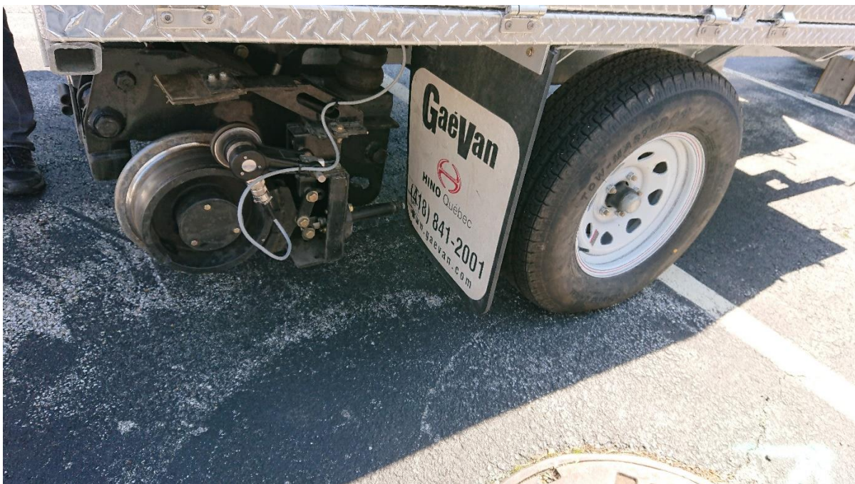
Figure 7 - Optical Encoder (Attached to Rail Wheel)
