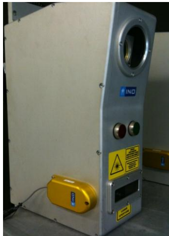
Figure 14. IMUs (gold) added to the LCMS sensors.
