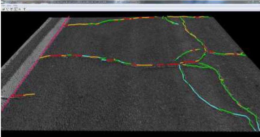
Figure 6. Example crack detection results (severity = color code).
