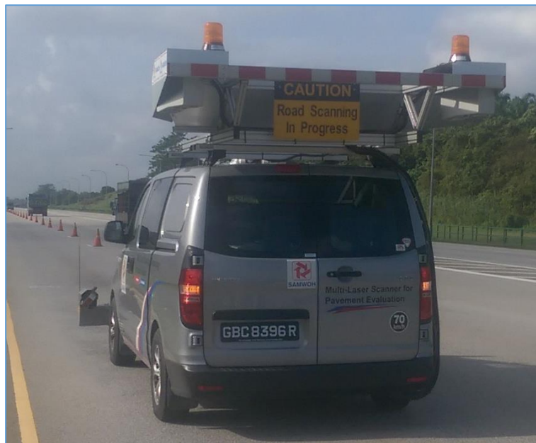
Figure 3: Vehicle with LCMS Sensors
