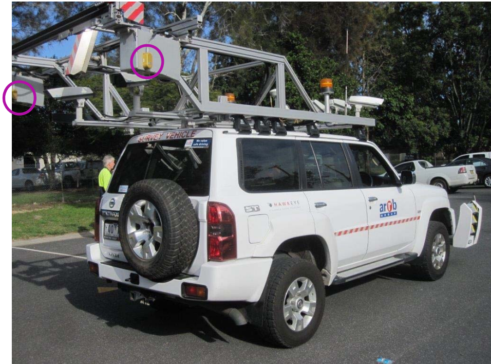
FIGURE 1 3D system with additional accelerometers (circled).
