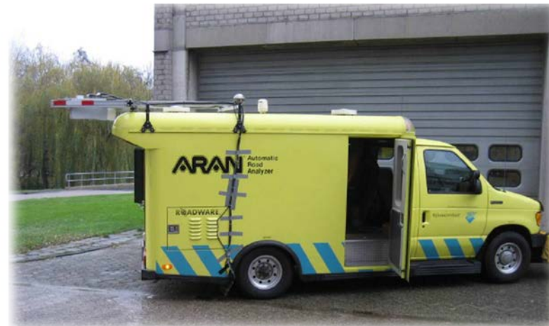
RWS ARAN 2 equipped with the LCMS system
