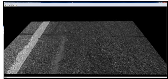
Figure 10: 3D image of ravelling produced by ACD (picture courtesy of Pavemetrics)
