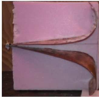
Figure 29 UWB horn antenna with foam supporting the structure.
