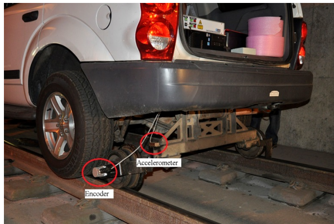
Figure 112 Installation of wheel encoder and accelerometer.
