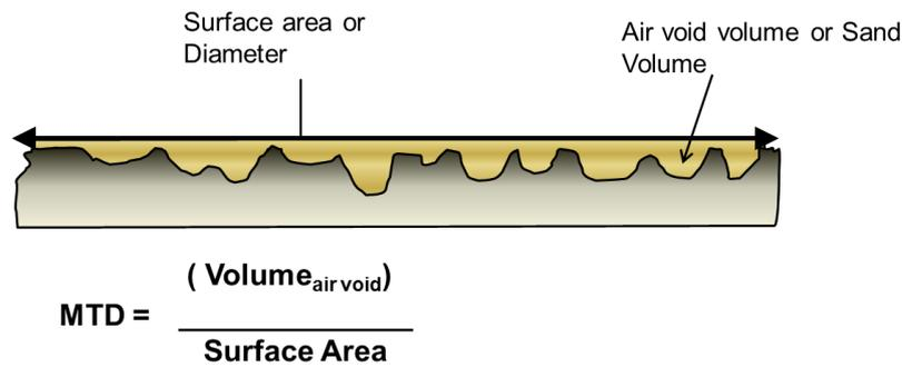
Figure 5. MTD calculation (Digital Sand Patch Method)
