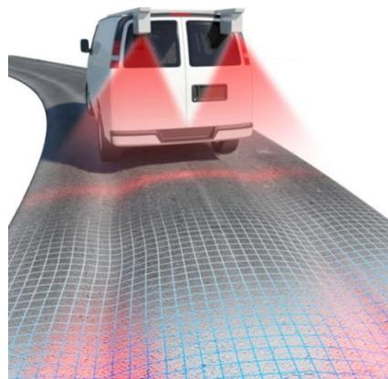
Figure 1. LCMS on an inspection vehicle.
