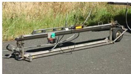
Figure 6. SLP (Stationary Laser Profiler)
