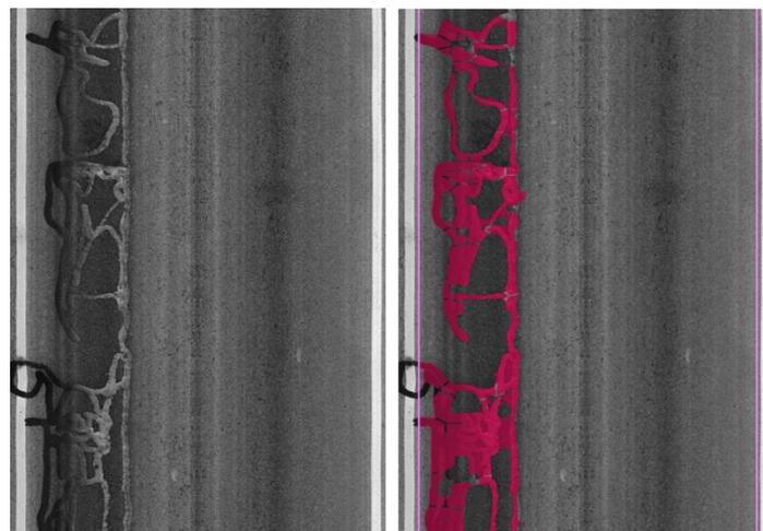
Figure 14. Example result of sealed cracks detection
