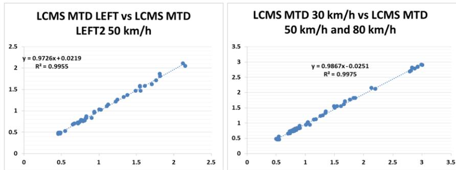
Figure 11. Repeatability of MTD texture values (multiple runs) of the LCMS at 50km/h (left graph) and 30km/h, 50km/h and 80km/h (right graph).
