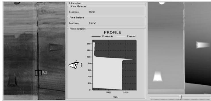
Figure 12. High gap (> 50mm) between dislocated and uplifted segments.
