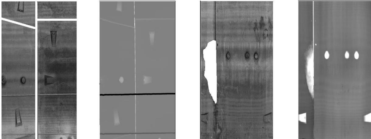
Figure 10. Common defects (I). The first two pictures show joints between assembled segments and the second two show surface chipping.
