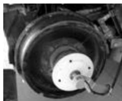
Figure 4. High-resolution odometer installed on the wagon's wheel.
