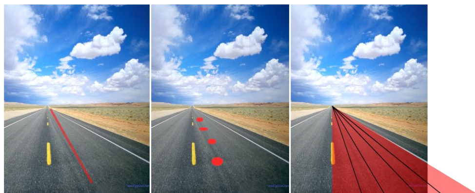
Figure 5. MPD (left), sand patch - MTD (center), LCMS - RPI (right)
