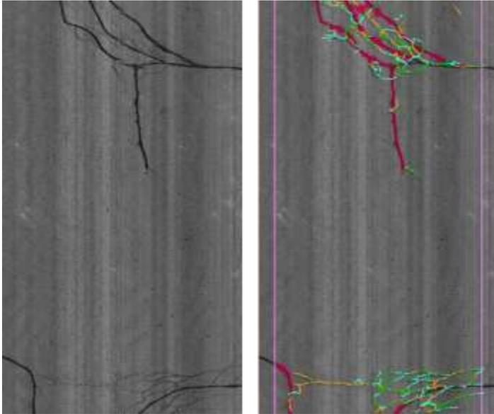
Figure 3. Three examples of sealed cracks detection on road surfaces (results in red)
