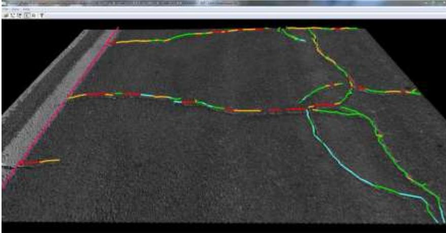
Figure 6. Example crack detection results (severity = color code).
