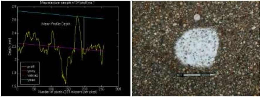
Figure 4. MPD vs sand patch.
