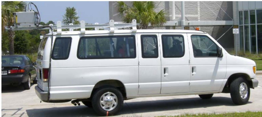
Figure 2 The sensing van for collecting faulting data.
