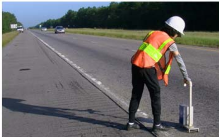
25 (b) Manually measure faulting on the roadway
