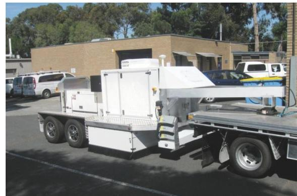
Figure 1: RoadCrack system – new trailer version
